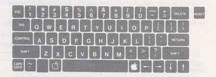
The Apple IIe keyboard is laid out like the most widely used electric typewriter keyboards, and now has 63 keys. Here are the new keyboard's features:
