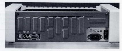
The Apple IIe has a metal back panel with 12 rectangular openings instead of the notches found on the Apple II and II Plus. This new back panel features small diagrams of the devices you can attach to each of the four built-in connectors, and specially arranged openings for disk drive cables, 9-pin and 25-pin D-type connectors.
